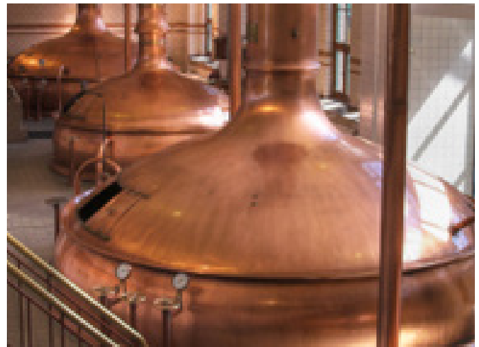
Polyclar Brewbrite wort clarifier and beer stabilizer is added to the kettle 10 minutes before the end of the boil.
